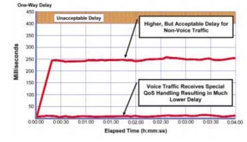
Figure 14. Segregating Packets by Delay Characteristics
